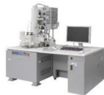
FE-SEM Morphology + Elemental Characterization
