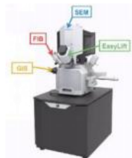
FIB Nanothin Sectioning
