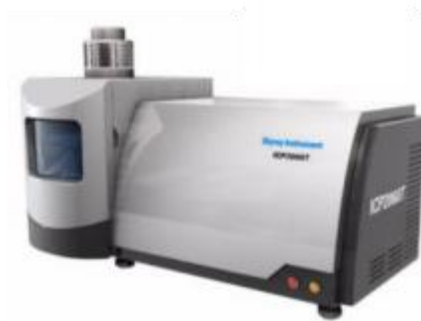
ICP-OES Compositional Characterization
