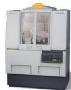
XRD Physical Phase Characterization
